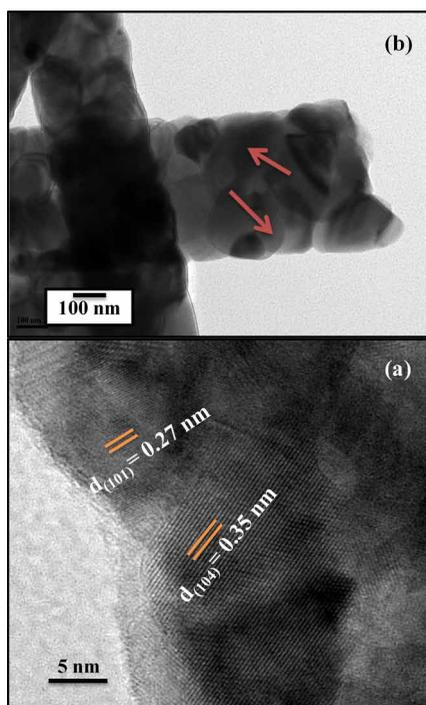
with the nanofibers. Upon closer inspection of the microstructure of these particles by HR-TEM, the presence of crystalline  $\text{CoTiO}_3$  with  $\text{TiO}_2$  (Figure 4b) has been confirmed. For  $\text{CoTiO}_3$ , the interatomic spacing of the lattice plane (104) was found to be 0.27 nm; whereas for  $\text{TiO}_2$ , the spacing for the lattice plane (101) was 0.35 nm.
